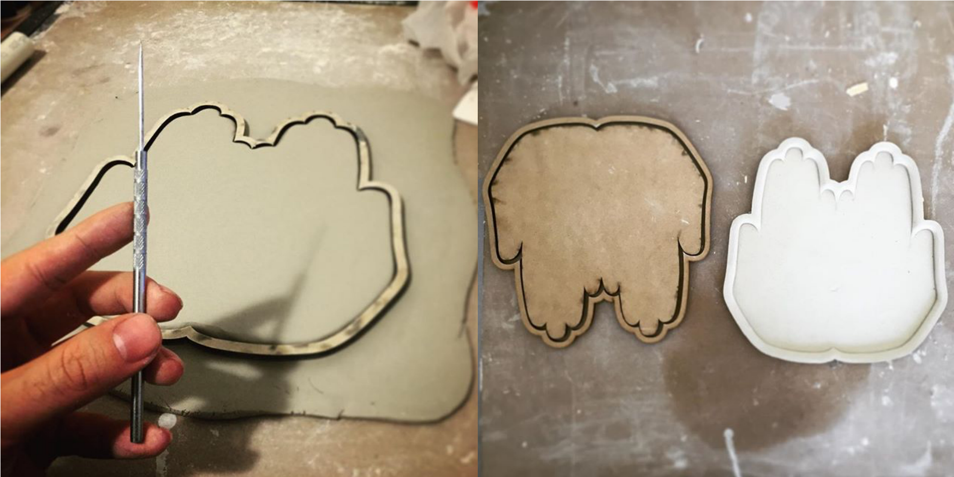
Adam Chau Laser cut molds used to create shallow trays
