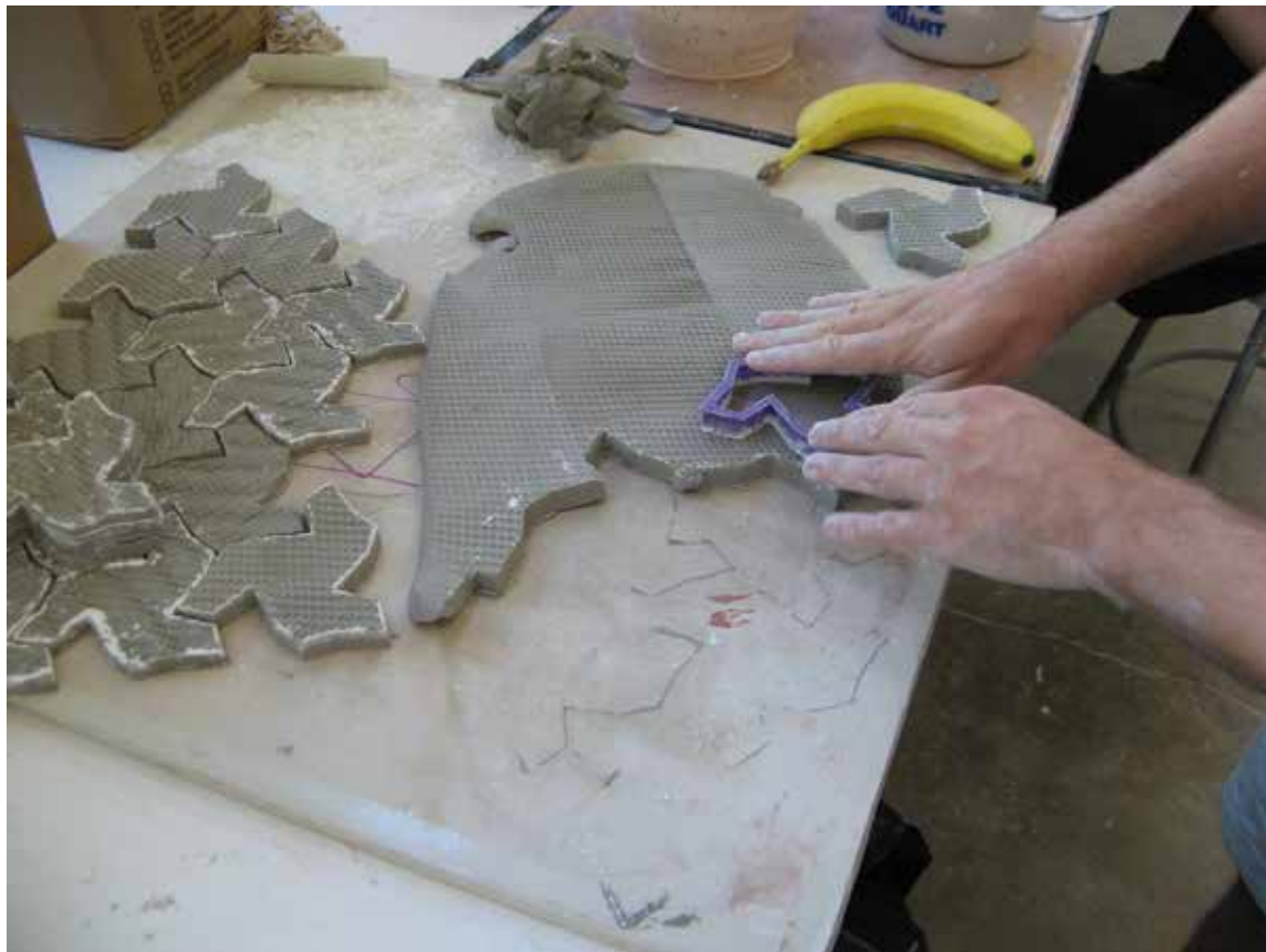
Jo Kamm's digital fabrications class at KCAI Bisqued terra cotta tiles Detail of the 3D printed tool used to make tiles
